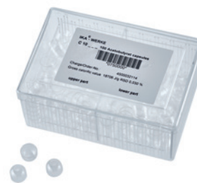
C 10 Acetobutyrate capsules 100 pieces; with known calorific value; to fill in samples with volatile compounds; not hygroscopic Ident. No. 0000750000
